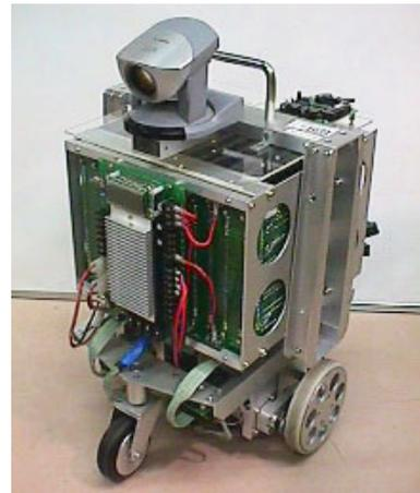
Fig. 1. Wheel Based Mobile Robot
