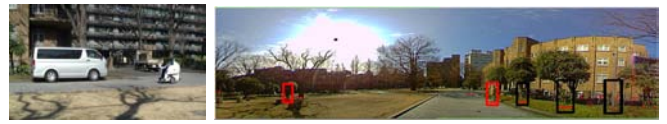
(a) Human detection result (red rectangles mean positive , black ones mean negative )
