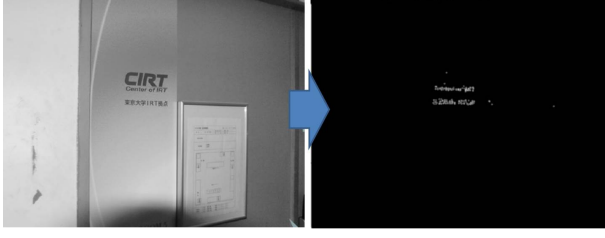
Fig. 6. Detection of character candidates by means of image frequency filtering. A group of white pixels show the region.
