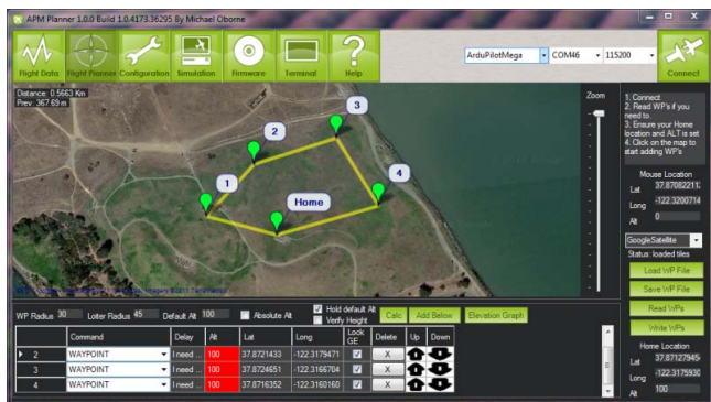
Fig. 2: Screenshot of GPS-based way point navigation based on ArduCopter software package. ( http://code.google.com/p/arducopter/ )
