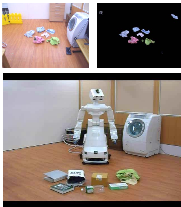
Fig. 1: Clothing detection results. Top left: input image, top right: detected clothing region. Bottom image shows an experiment that a robot sought an item of clothing from cluttered floor.
