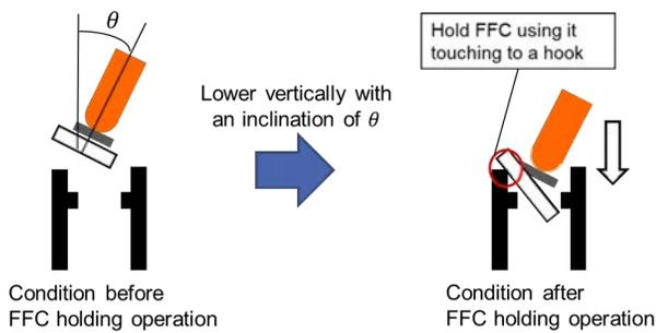
Fig. 4. The motion procedure(1) of wiring of hook No.5
