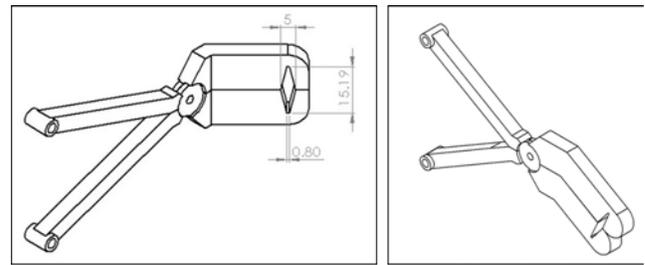
Fig. 6. End-effector design (left: for FFC operation, right: for FFC folding)
