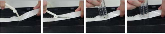
Fig. 7. Shapes of tip of end-effector: From the left, point grounding, spring, rectangular, circular.
