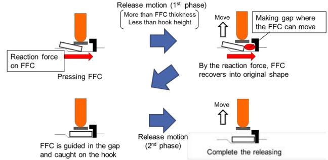
Fig. 3. Releasing action of FFC
