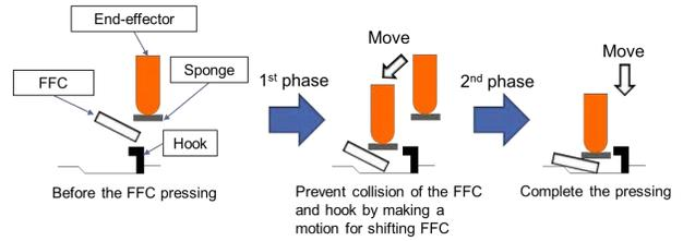
Fig. 2. Pressing action of FFC
