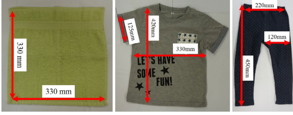
Fig. 4. The dimensions of target fabric products. Left: Towel, Center: T-Shirt, and Right: Pants.
